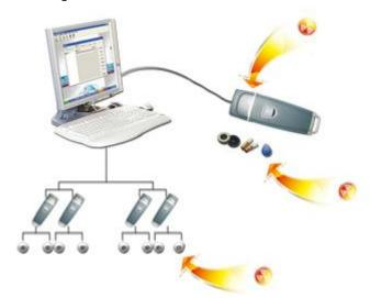
1. 5000V5 reader 2.POGO Pin connecting cable 3.Charger 4.RFID tags 5.Guard ID card 6.Management software
